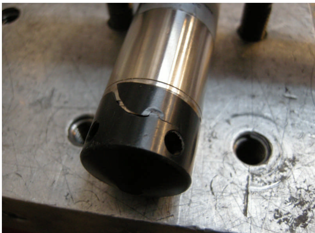
Photo 8. Impact (level sensor after impact).
