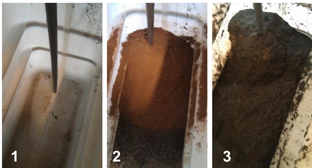
Figure 2. Photo 1 shows the LevelTec pressure sensor installed in the small scale slurry container used for the performance test. Photo 2 shows the LevelTec sensor covered by sand. Photo 3 show how the sand is placed around the LevelTec sensor after the slurry container was filled with slurry and emptied again. It is seen that the sand is still laying around the sensor.
