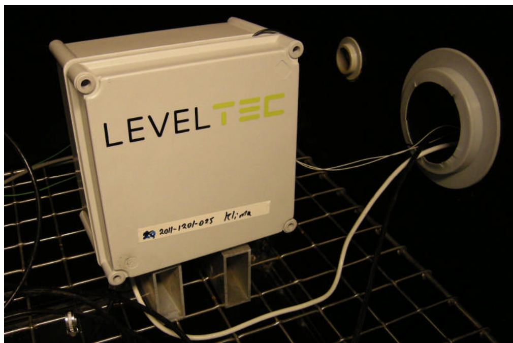
Photo 1. Climatic tests; dry heat, cold and humidity (control unit).
