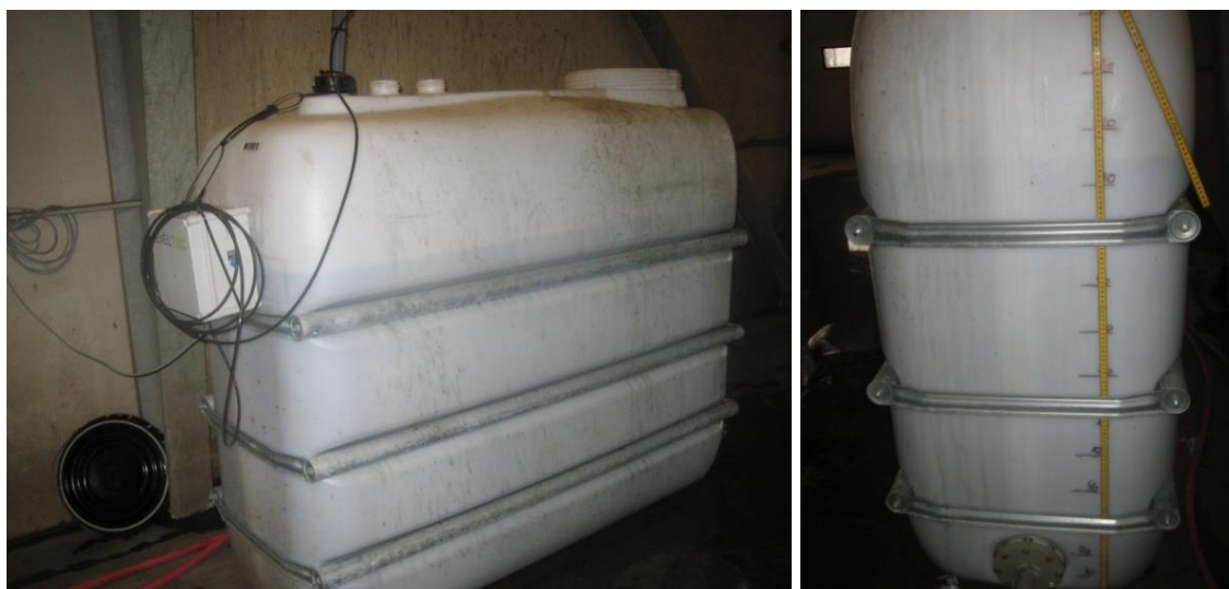
Figure 1. The small scale slurry container used for the performance test of LevelTec. On the left photo the LevelTec control unit is seen as a grey box installed on the end of the slurry container.
