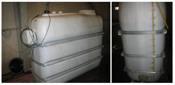
Figure 5. The small scale slurry container used for the performance test of LevelTec. On the left photo the LevelTec control unit is seen as a grey box installed on the end of the slurry container.
