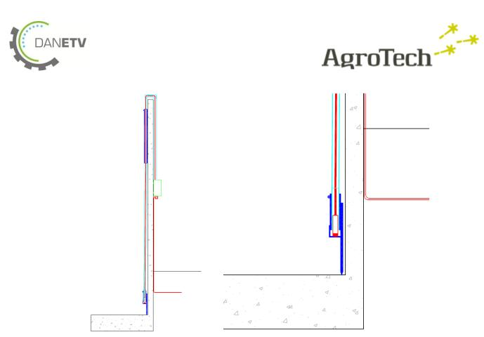
Figure 3. To the left is shown a cross section of a slurry storage tank with LevelTec installed on the tank wall. A PVC tube is mounted on the inner side of the tank wall (light blue). The pressure sensor (drawn in red colour) is placed inside the tube and lowered to a position approximately 0.20 meter above the bottom of the tank. To keep the pressure sensor in a fixed position a stand is mounted at the end of the PVC tube. The stand is shown in dark blue colour on the right side of the figure.
