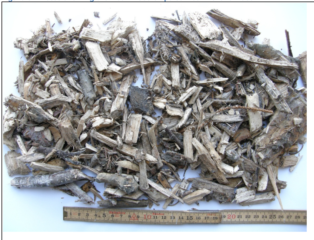
Figure 6. Photos showing the fresh wood chips burned in the furnace
