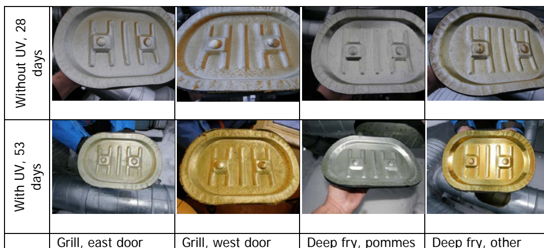
Figure 5 Inspection doors – with and without JIMCO KPC system switched on
