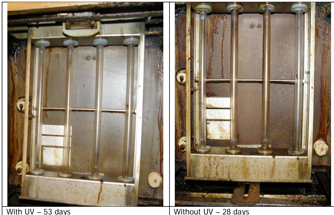
Figure 7 Deposit on one wall section.
