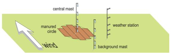
Figure 4. Layout of a circular plot for the measurement of NH3 volatilization using the micrometeorological mass balance method, with masts supporting NH3 traps at various heights in the center of the plot and at the windward boundary of the plot. Source: VERA Secretariat, 2009 [2].
