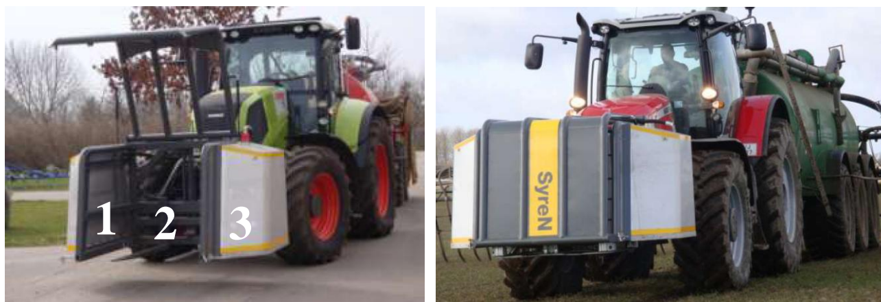
Figure 1. The SyreN-system includes three tanks installed on the front of the tractor. 1: Tank for iron sulphate. 2: Here the tank for sulphuric acid shall be placed. 3: Tank for water for cleaning the system.
