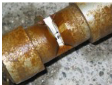
Figure 3.2 Effectiveness of hydraulic-pneumatic cleaning of measuring windows.
