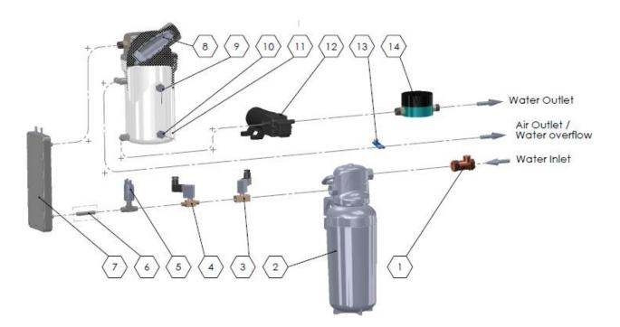
Figure 2.2 Process diagram: 1: DS EN/6117 Approved non-return valve; 2: Head and cartridge for filter/softener; 3 & 4: Solenoid valves; 5: Pressure switch; 6: Optional flow restriction; 7: BacTerminator® disinfection chamber; 8: Bio Reaction Zone; 9: Water tank with 20mm air gap; 10: Level sensors; 11: Pump; 12: Pulsation dampener; 13: Leak detector
